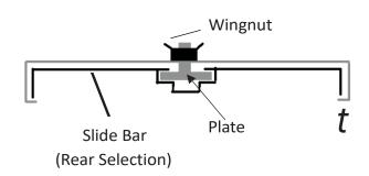
4. Fix the fishtail adaptor into the opening on the slide bar.
