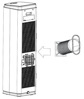
4. Make sure the unit is upright, and there are no obstructions to the air inlets and outlet grills, with at least 50cm of space to the sides and rear of the unit.
